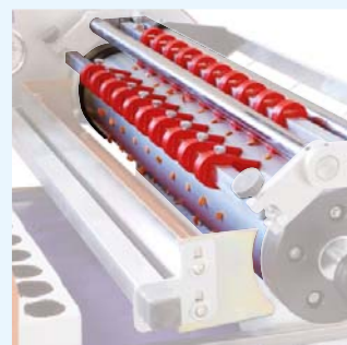
13 Air bars with labyrinths suitable to work with big seeds .
